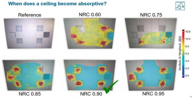
A color map showing sound reflecting off a mineral-fiber panel acoustic ceiling with an NRC rating of 0.60 (yellow).
